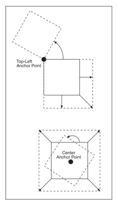
Figure 7.12 How an anchor point should affect scaling and rotation of a sprite
