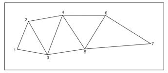
**Figure 7.9** A triangle strip that defines five triangles using seven vertexes.
