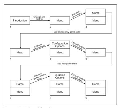
Figure 10.2 A stack-based state system
