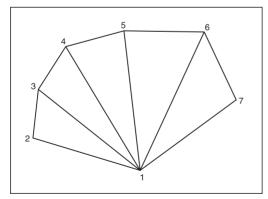
**Figure 7.10** A triangle fan that defines five triangles using seven vertexes.
